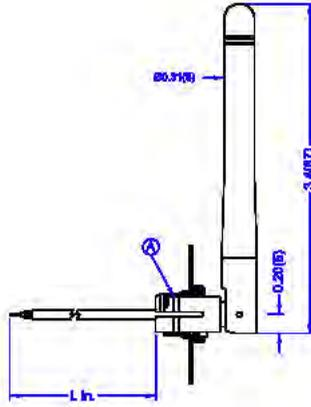
(April 09, 2009, Fairfax, Virginia) Nearson Inc. will be releasing a new antenna series with their second generation click mount hex bushing, which adapts to electronic products whose enclosure walls are constructed of thicker than usual material.
